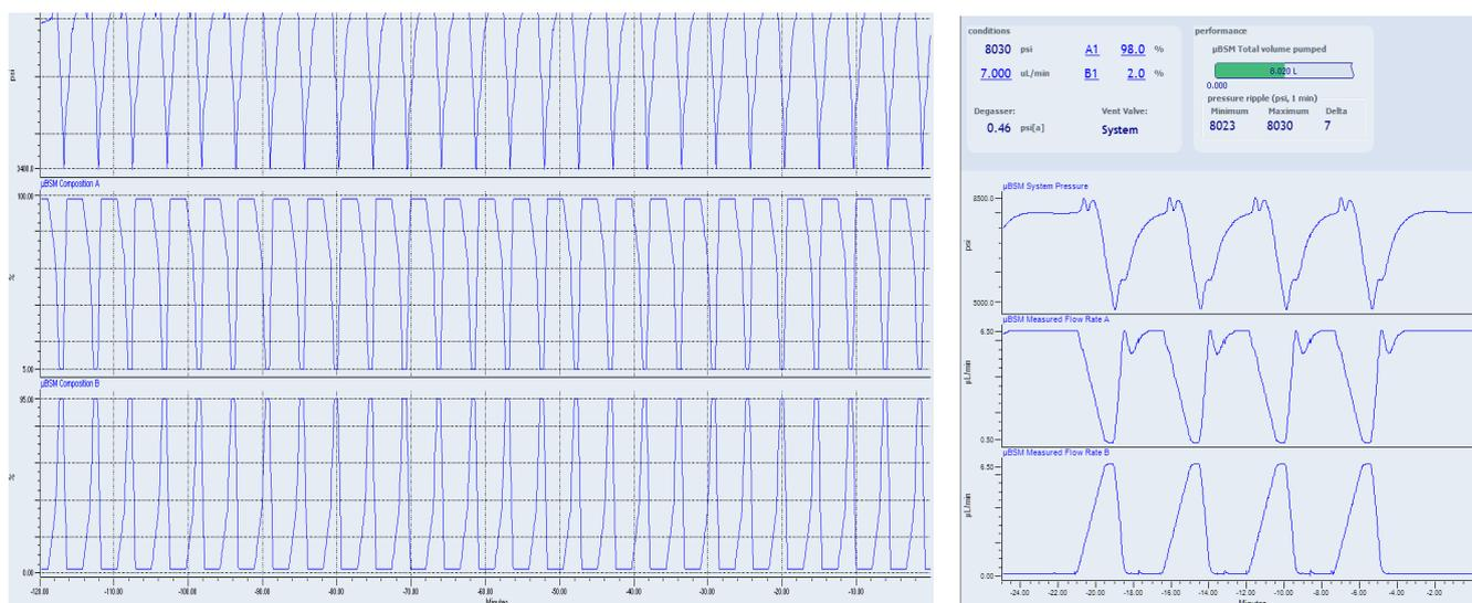
**Figure 2.** A screen capture of the ACQUITY UPLC M-Class Binary Solvent Manager showing system pressure change during sample analysis. On the left is the pressure history using the HSS T3 iKey in a two hour period, and on the right the system pressure using the BEH iKey for four sequential injections. In each graph, the top trace is the system pressure, and the middle and bottom traces are composition changes in channel A or B, respectively.
