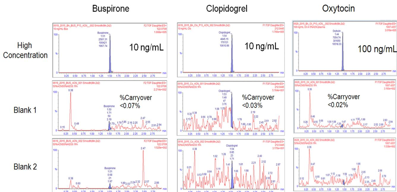
**Figure 3.** Chromatograms from the carryover study of the three compounds. The top chromatograms for each compound are from sample injection, followed immediately by blank injections reflected in the middle and lower chromatograms. Compound-specific gradient conditions were used.
