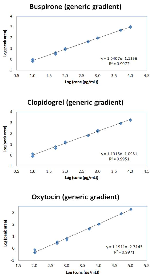
**Figure 6.** Plot of peak area versus concentration for serially diluted solutions of test compounds in human plasma. Each concentration was injected in triplicate and plotted. Generic gradient conditions and a scan rate of 0.036 s were used for all compounds.
